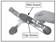
Figure 7. Installing guard.
